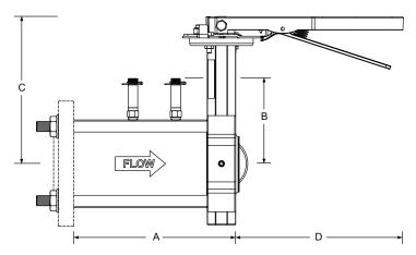
Model AF Shown with Customer supplied Outlet Companion Flange (In Dashed Line), Threaded Rods, Washers & Nuts are supplied.
